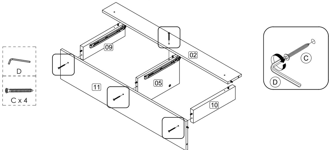
**Step 4:** Attach bottom panel (2) to side plate (9) and (10) using hardware G with a screwdriver (not provided).
