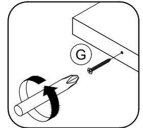
**Step 6:** Hit hardware H into bottom of side panel (3), (4) and leg panel (16).
