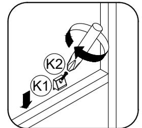
**Step 10:** Insert hardware I into mounting positions on side panel (3) and center panel (5).
